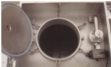
FIGURE 33: Pressure inlet with pneumatic valve
