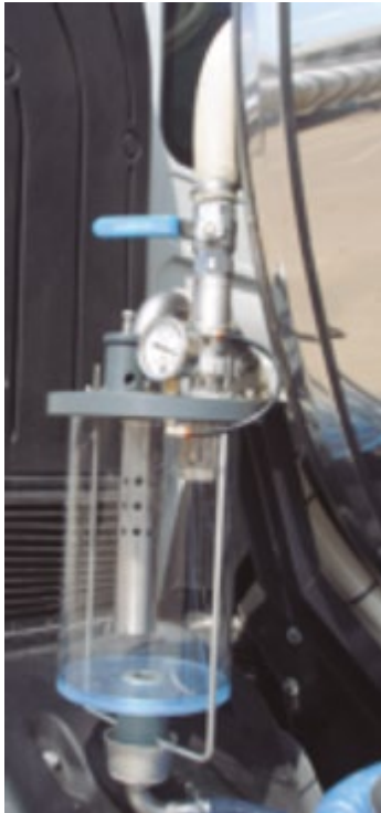
FIGURE 36: Vacuum vessel on a milk tank truck
