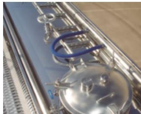
FIGURE 26: Airline with detachable flexible hoses
