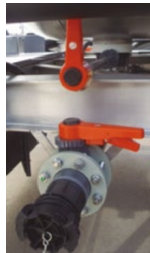
FIGURE 29: Plastic manual valves on ADR tank
