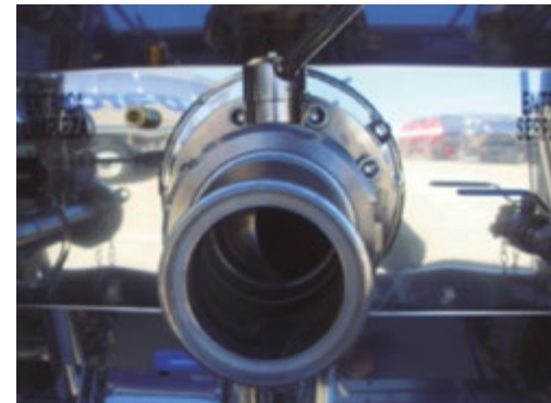
FIGURE 27: General manifold with manual outlet valve at rear
