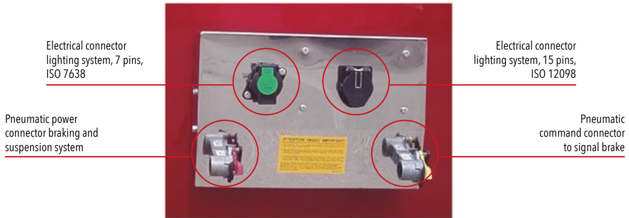
FIGURE 2: Electrical and pneumatic connections
