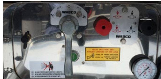
FIGURE 8: Brakes and suspension controls cabinet
