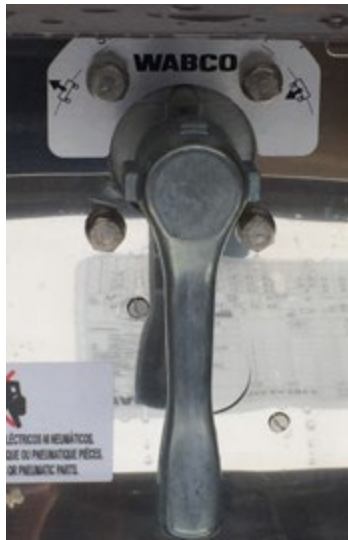
FIGURE 7: Suspension height control handle
