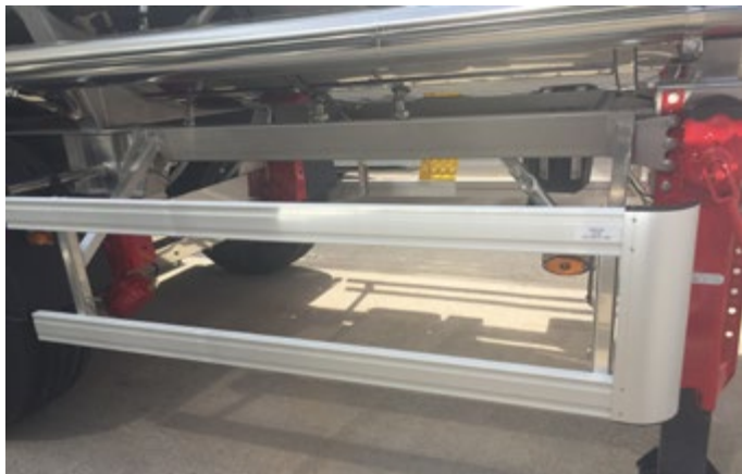
FIGURE 18: Side protections for cyclists
