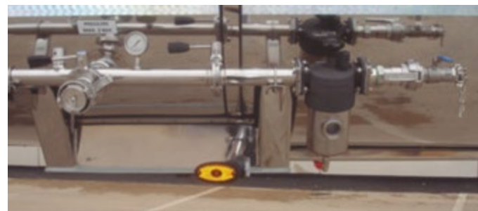
FIGURE 25: Pressure manifold with inlet filter
