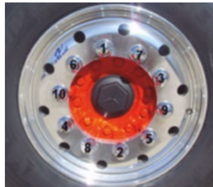
FIGURE 11: Tighten the bolts in star
