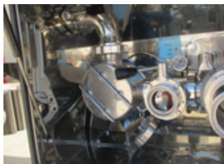
FIGURE 32: Self-priming pump with rubber impeller, hydraulic driven and overfill control
