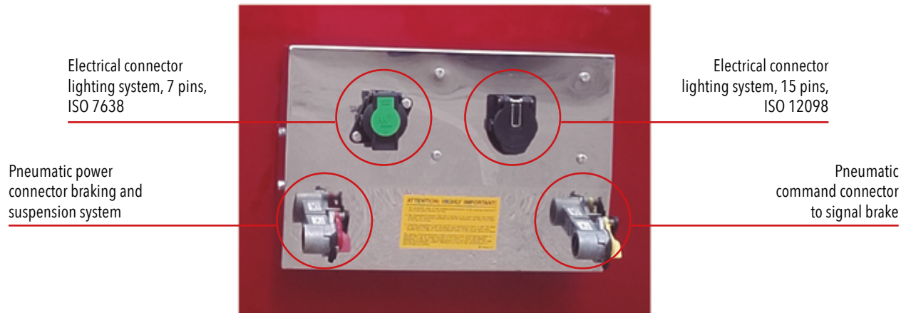
FIGURE 2: Electrical and pneumatic connections
