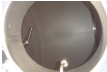
FIGURE 20: Inner cleaning shower with overflow sensor
