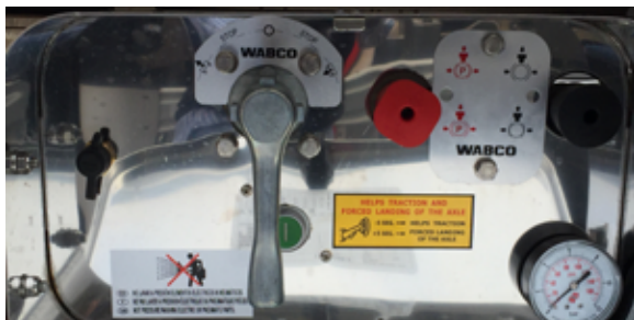
FIGURE 7: Brakes and suspension controls cabinet
