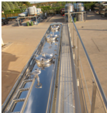
FIGURE 19: Top cleaning connection
