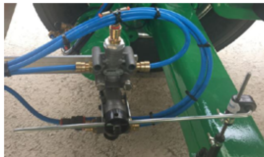
FIGURE 4: Levelling valve with cut
