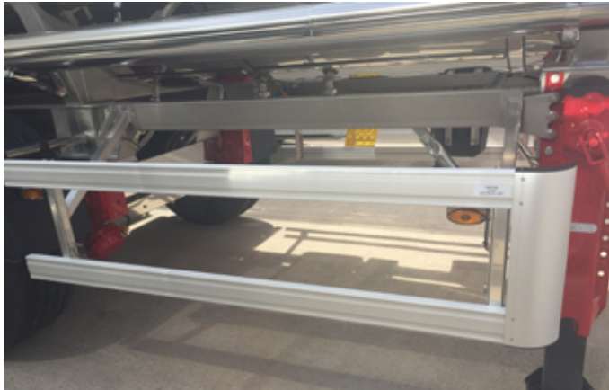
FIGURE 15: Side protections for cyclists
