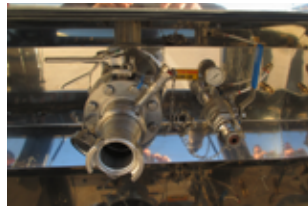
FIGURE 27: Manual valve with handle extension to be operated from one side
