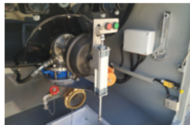
FIGURE 31: Example of discharge box in bitumen tank
